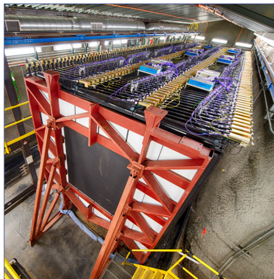
Near Detector 300 tons 16 m x 4.1 m x 4.1 m 214 layers, ~20,000 channels
