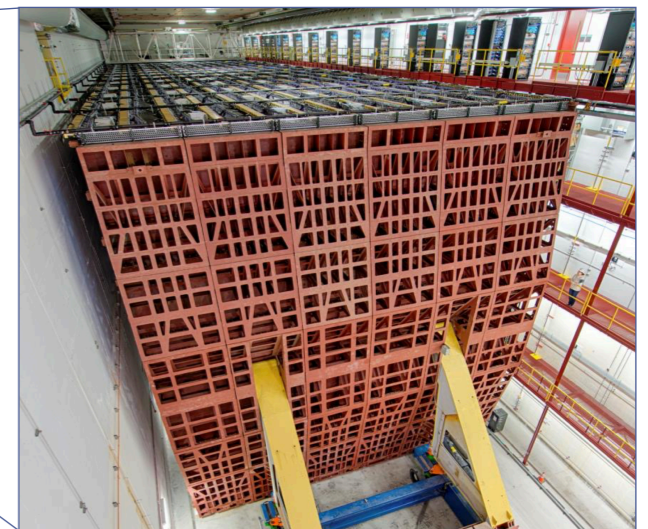
Far Detector 14 kton 60 m x 15.6 m x 15.6 m 896 layers, ~344,000 channels
