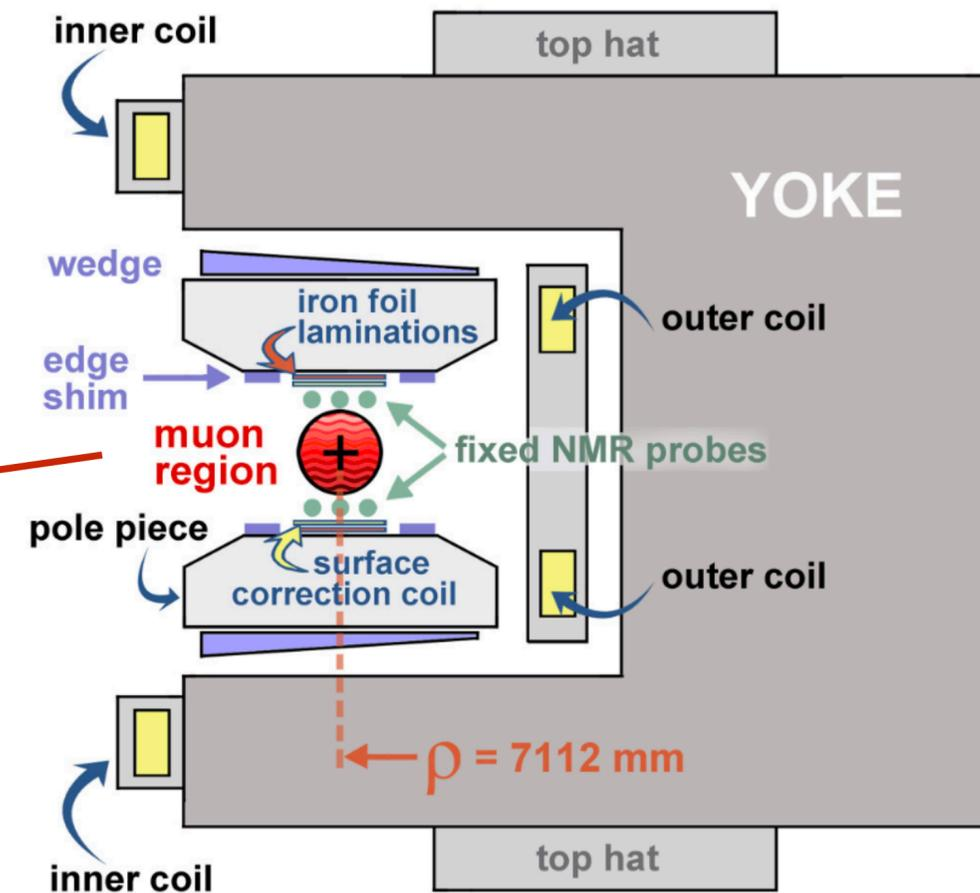
Gradients in muon region measured every ~3 days by a trolley with 17 NMR probes
