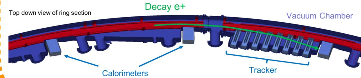
Muon precession frequency = frequency of number of electrons in detectors vs time
