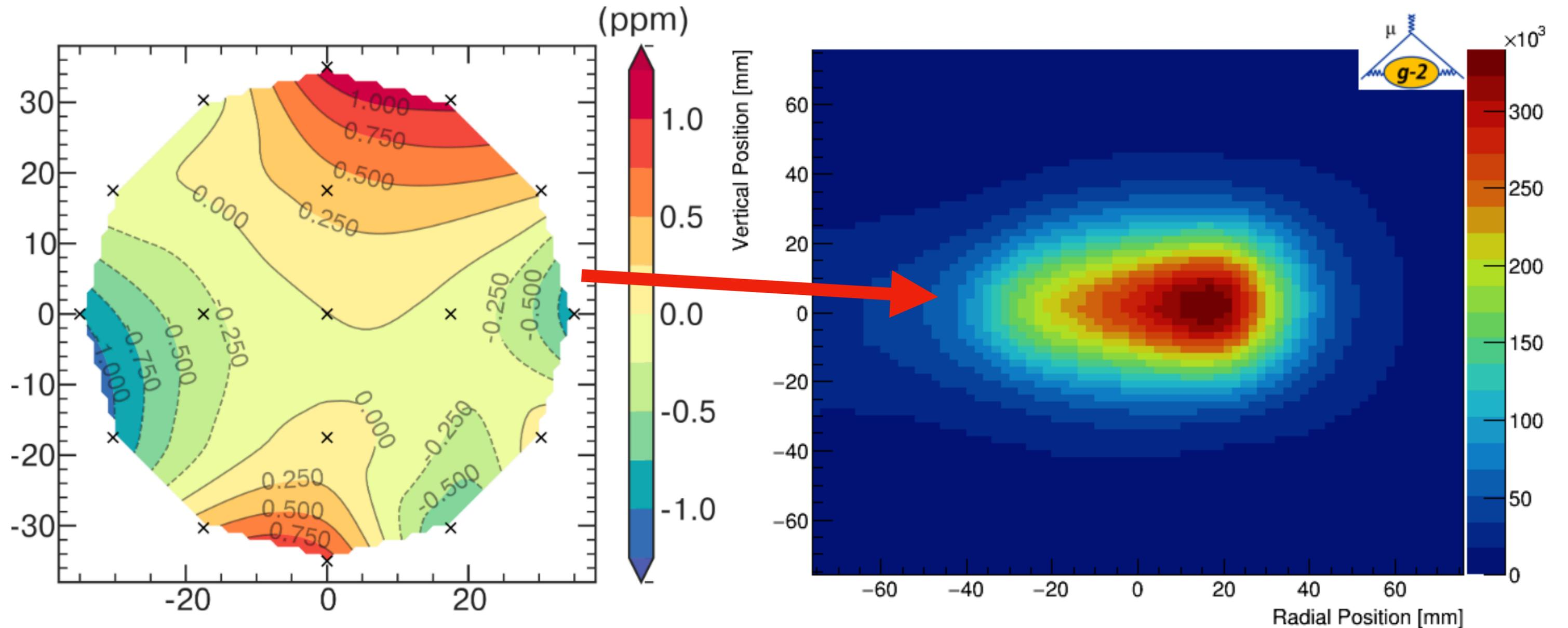
The muon beam does not sample all parts of the ring equally - some parts of the field are used more than others
