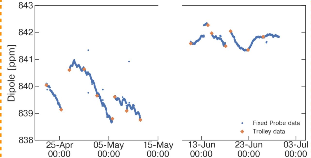
Relate trolley measurements to fixed probe measurements to obtain the field during the times the muons were present
