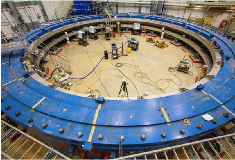
Muons orbit around the magnet and **precess**
