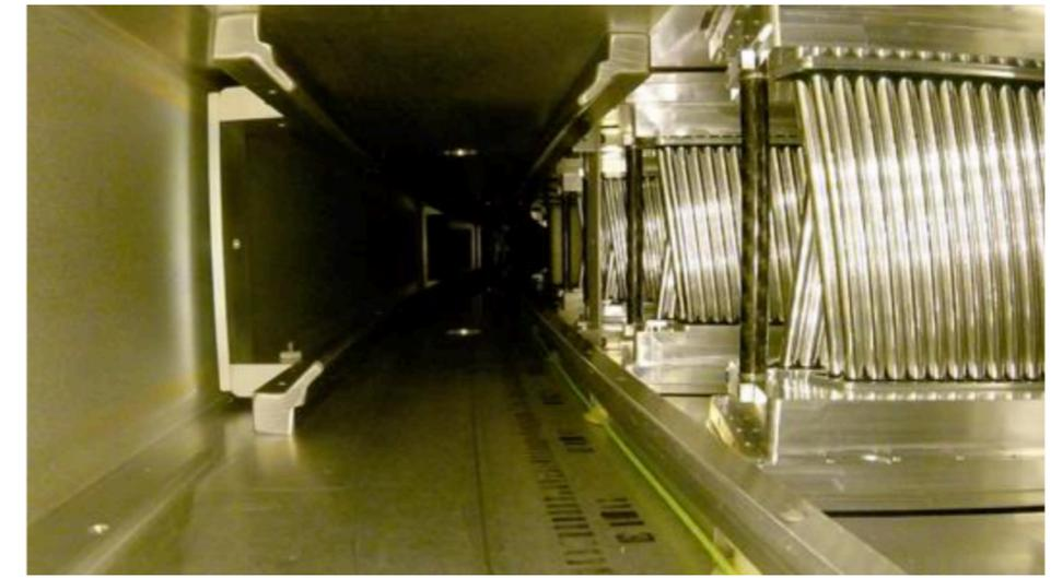
Straw trackers reconstruct muon distribution, determine complex beam dynamics
