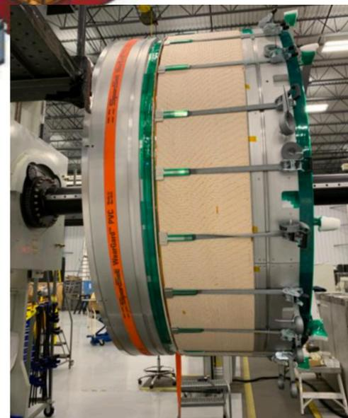
Coil layer compaction
