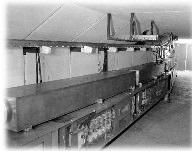
2 Test girders in village with 4 magnets
