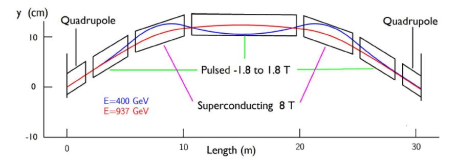
Pulsed dipoles first oppose, and later support the bending form 8 T superconducting magnets
