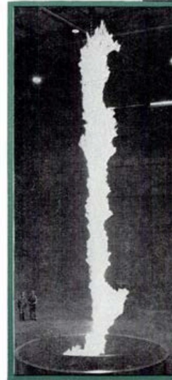
This 55-foot man-made arc was drawn out in Westinghouse laboratory in recent test.
