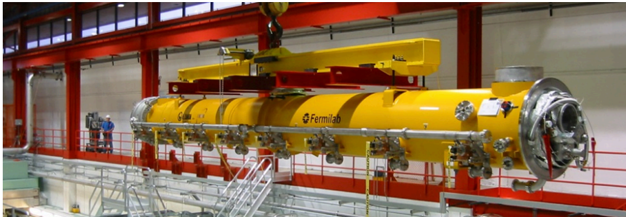
ILC cryomodule with record average gradient for FAST facility
