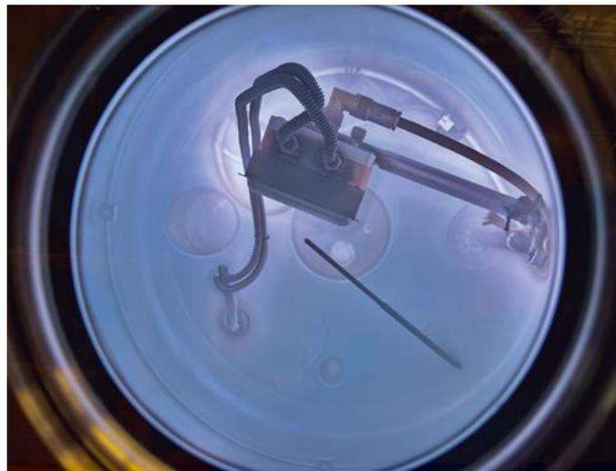
Vacuum Chamber Installed – Mirror Cleaning Facility at PPPL
