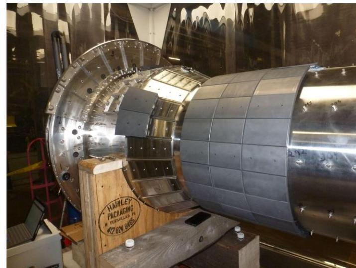
Scope: Fabricate In625 precision weldment = inner vacuum boundary
