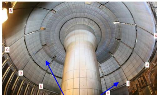
Discrete copper plates (Qty: 48), covered in tiles, mounted via in-vessel bracketry
