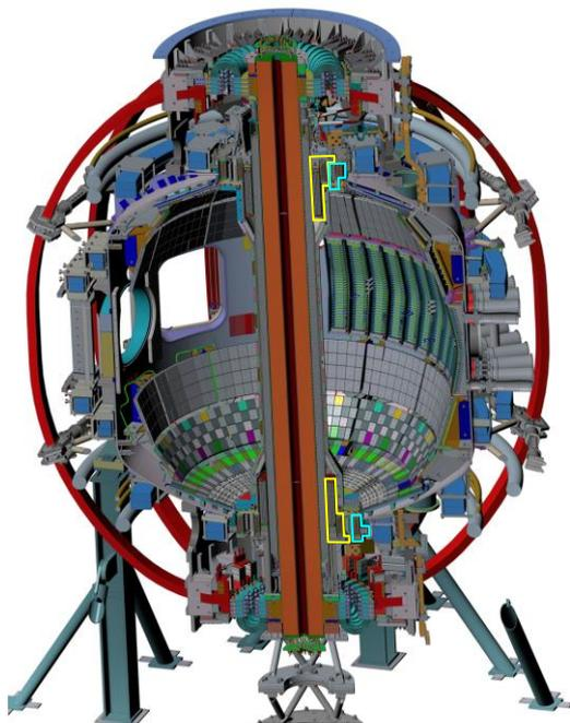
Scope: Fabricate & install 4 inner-PF coil supports
