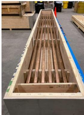
Gun Drilled Conductors
