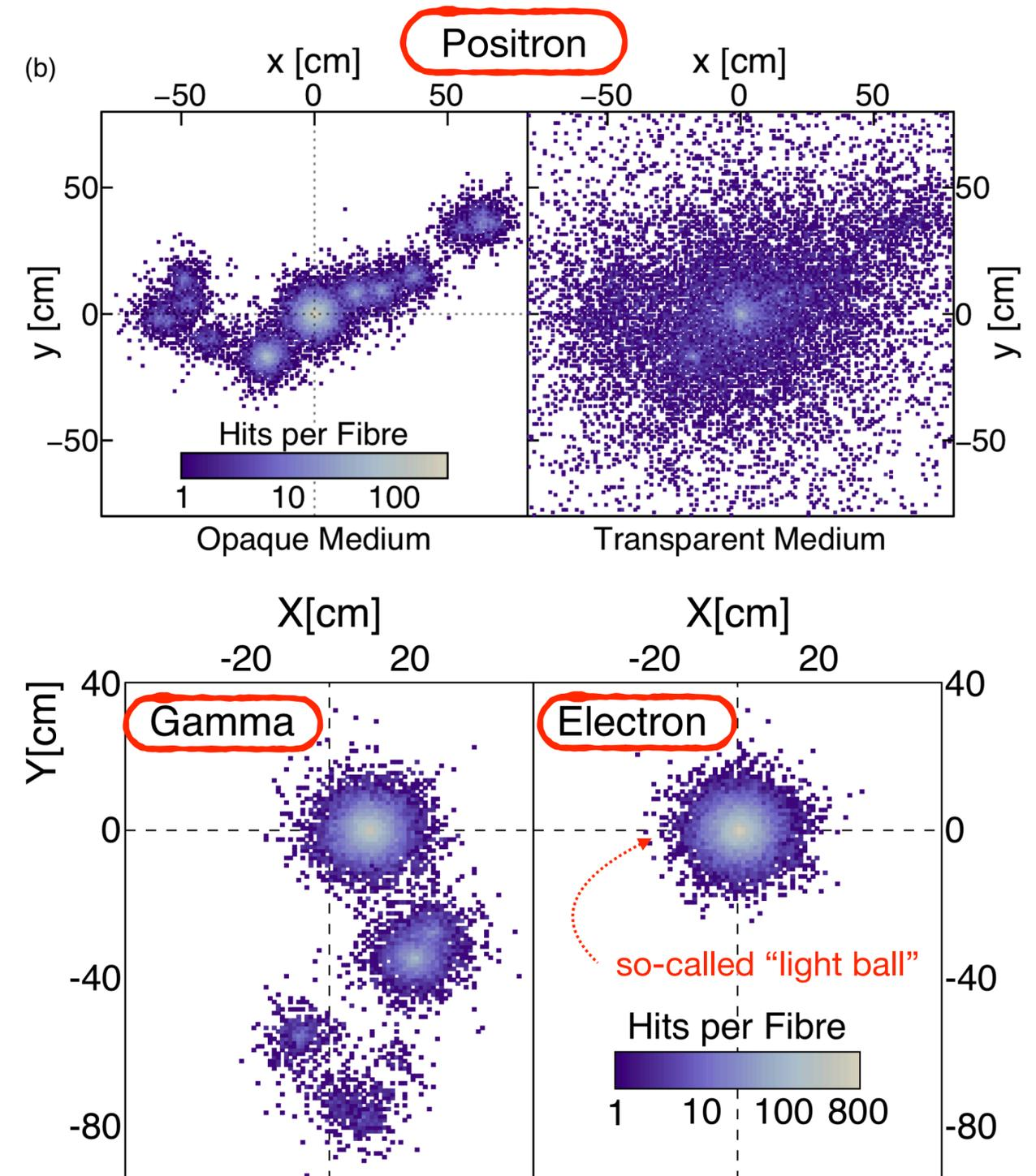
Each of these panels assumes a 1cm fiber pitch, one pixel per fibre, 2MeV of energy
