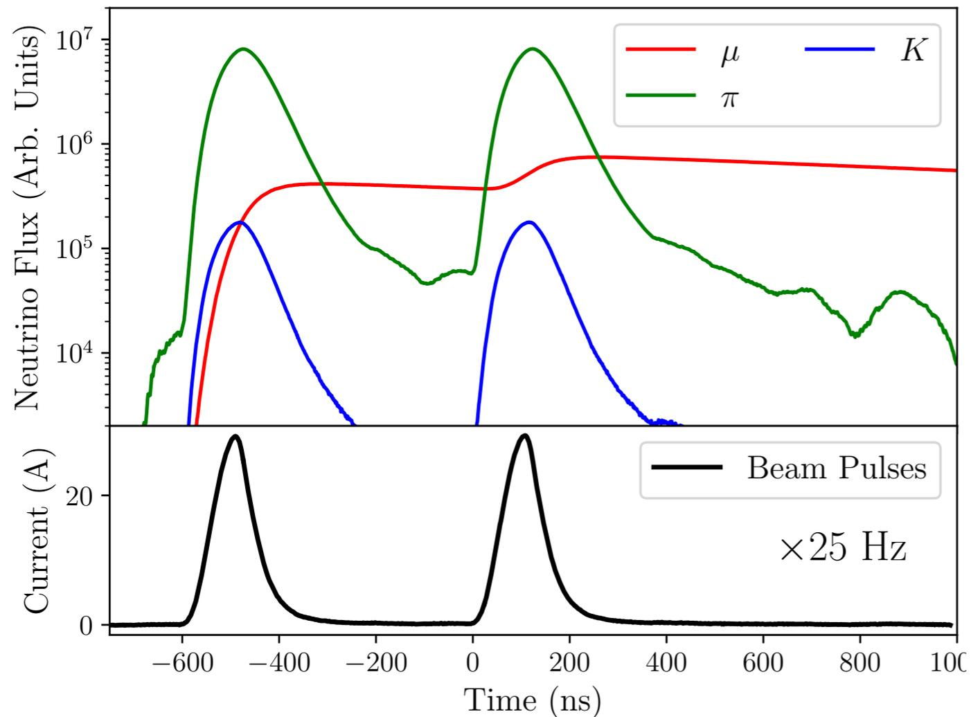
The J-PARC beam is delivered in two close pulses at 25 Hz, producing “prompt” (pion and kaon) and “delayed” (muon) neutrinos.
