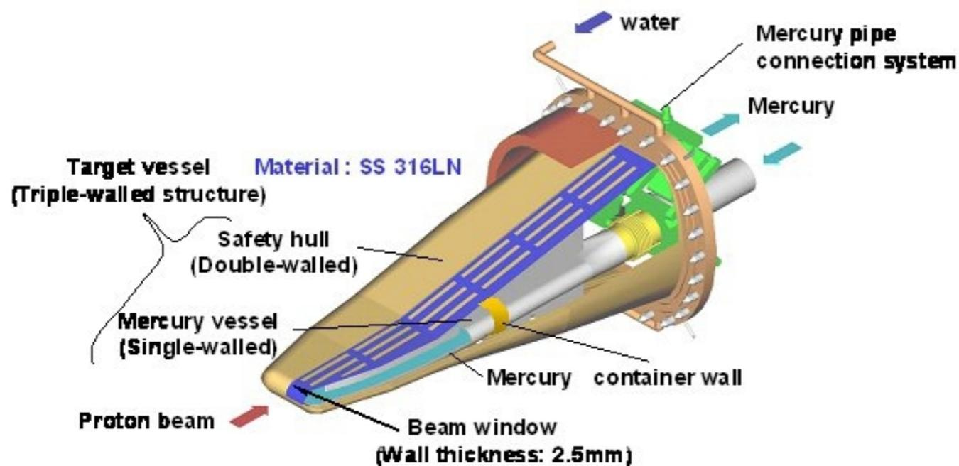
Neutron/neutrino production target is a double-walled SS vessel with circulating mercury.
