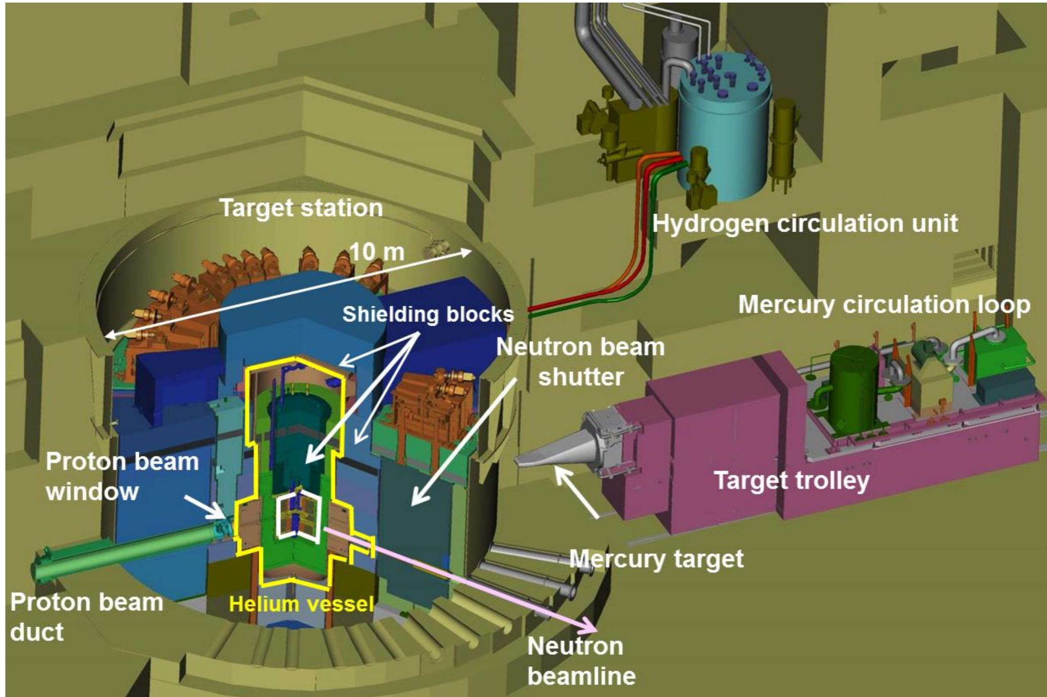
3 GeV protons on a mercury target @ 830 kW
